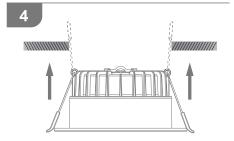
Fit the fixture in the ceiling by lifting the spring clips upwards.
