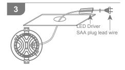
Cut out a hole in the ceiling. Ensure there is sufficient clearance in the area where you will be positioning the fitting. Choose the prefered colour temperature via the switch on the controller.
